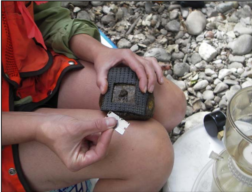
Figure 26. Template method used for scraping algae from stream substrate.
