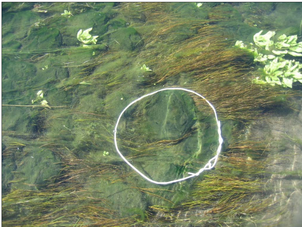
Figure 23. Sampling algae in Thompson Creek using the hoop method in 2009.
