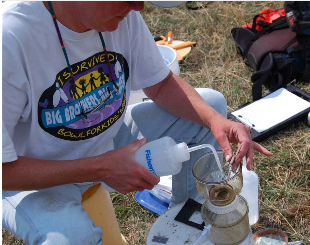
Figure 22. Filtering algae scraped from a sampled rock.
