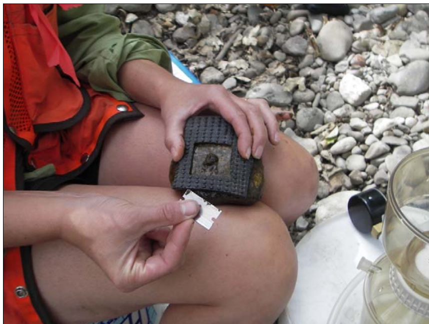
Figure 21. Template method used for scraping algae from stream substrate.
