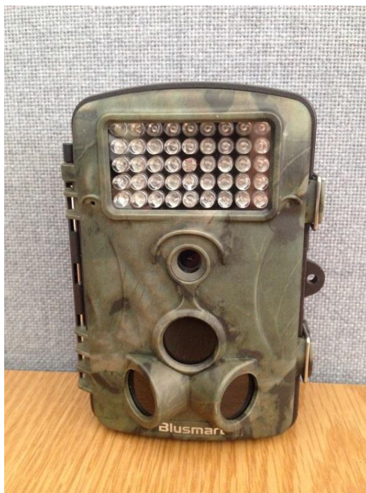
Figure 2-1. Camera used to photograph the staff gage on Ashley Creek downstream of Ashley Lake
