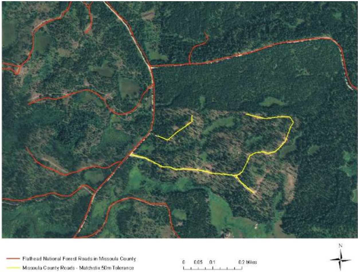
Figure 18. Example of unique segments from MatchStix output using 50 meter tolerance. Note how the smaller Missoula County segment does not intersect with the FNF segment
