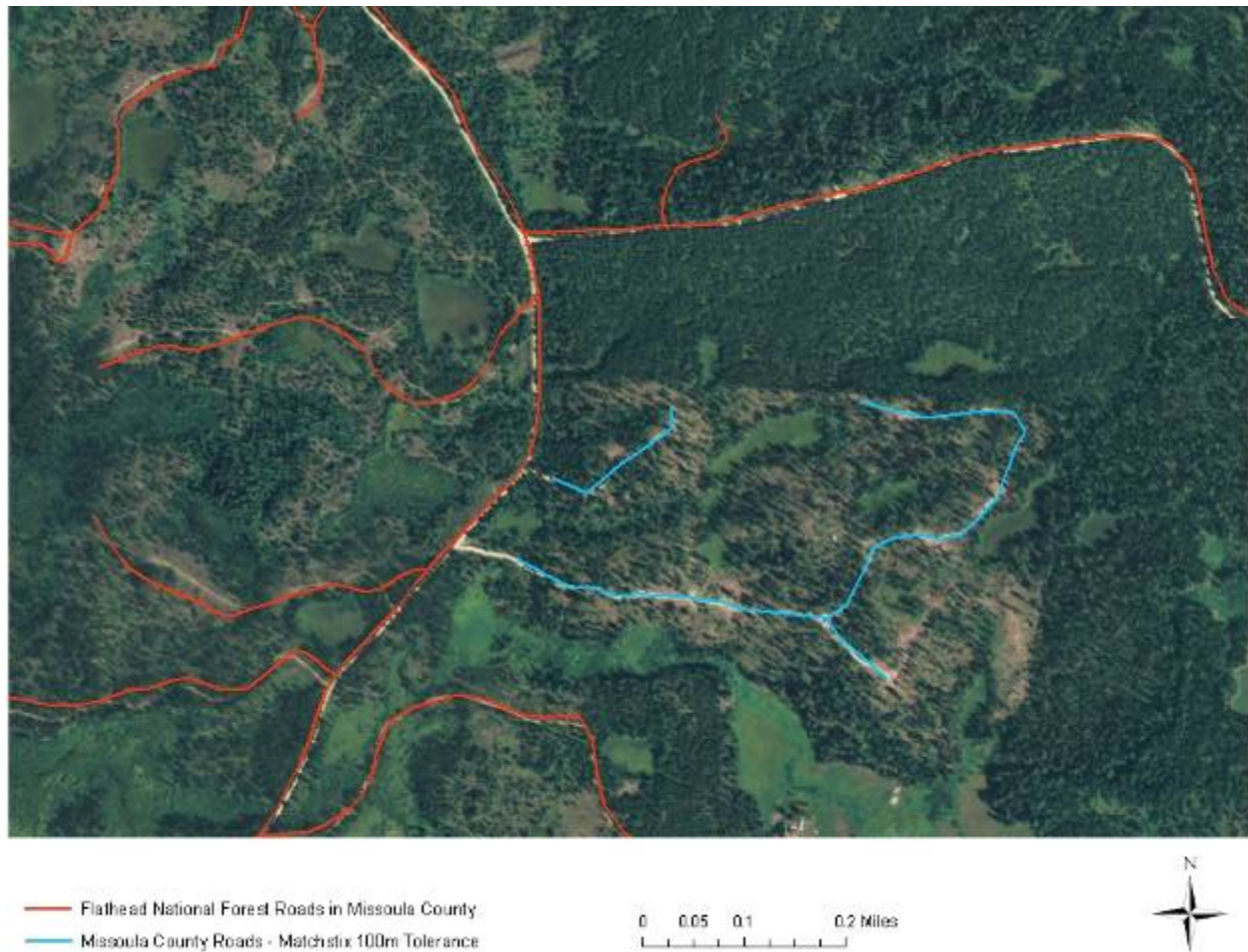
Figure 19. Example of unique segments from MatchStix output using 100 meter tolerance. Note how both Missoula County segments do not intersect the FNF segment
