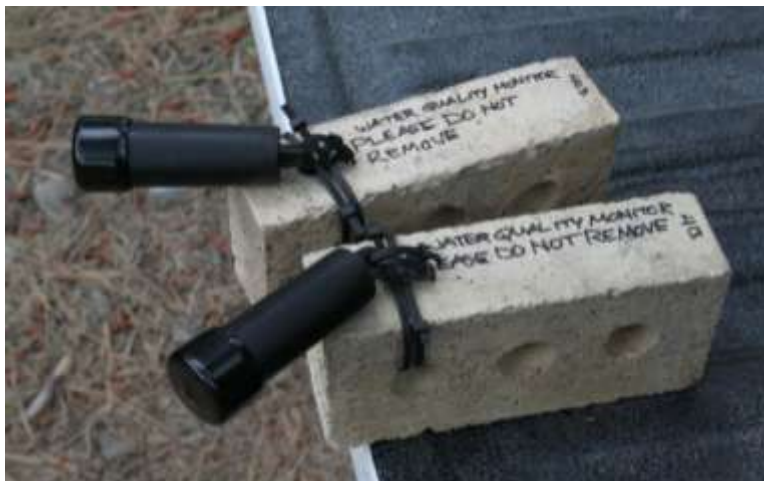
Figure 7. HOBO Pro v2 Temperature Data Loggers ready for deployment.
