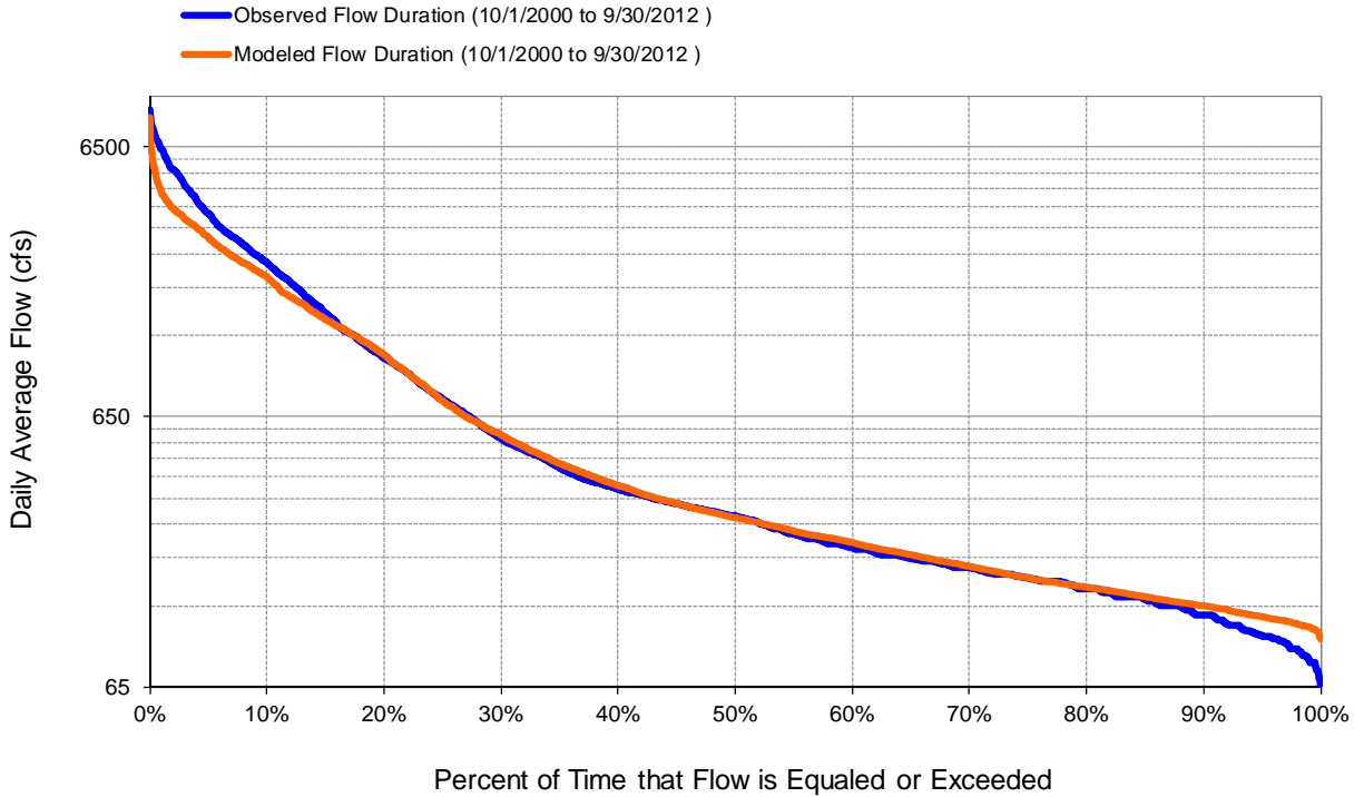
Figure G-1. Calibration Observed and Modeled Flow-Duration, USGS 12355000 Flathead River at Flathead, BC
